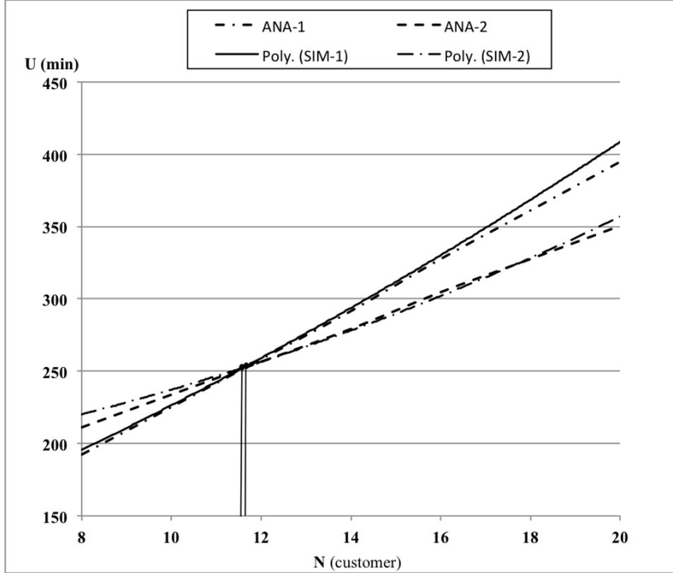
Figure 3.2: Utility function curves for one-vehicle case and two-vehicle case
